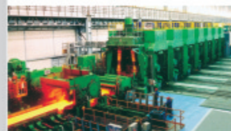
精轧机 Finishing mill
